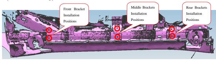
Step 3: Install the side bar on the brackets and then adjust the side bar to the proper positions.
