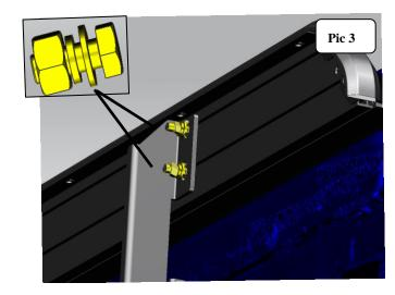
Step 4: Refer to Pic 3 to install V1 Running Board with running board hard ware.
