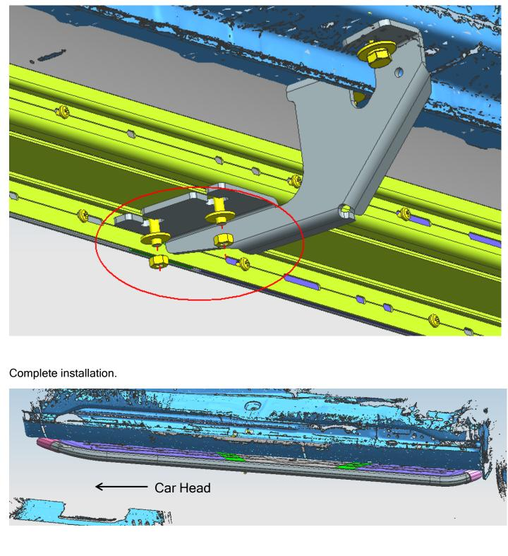
Step 3: Attach running boards on the brackets with Hex nuts M6 and Flat washers D6.
