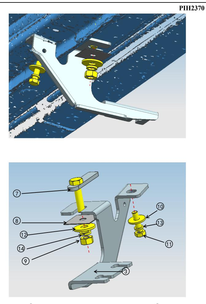
Rear Bracket (L) (5) is installed as below figure shown, Rear Bracket (R) (6) are in symmetrical **1-866-926-2867** | **39 St. Mary's Place, Freeport, NY 11520** | www.blackhorseoffroad.com
