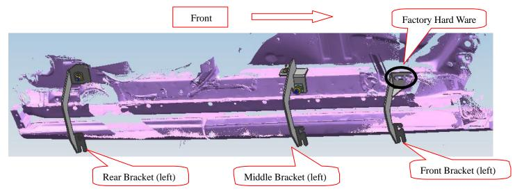
Step 3: Install the running board on the brackets and then adjust them to the proper positions.
