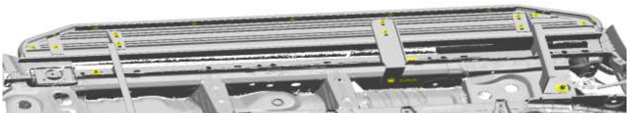
(Fig 5) Install running board and tighten all the standard parts
