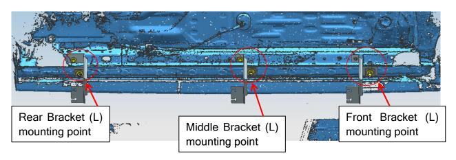
Step 2: Attach Front Bracket (L) ①, Middle Bracket (L) ③ and Rear Bracket (L) ⑤ on the mounting points with T Bolts M10x40⑦, Plastic Retainers $\phi$ 10 ( $\delta$ 0.7\*40\*40)⑧, Hex Nuts M10⑨, Flat Washers D10 (10x30x2.5mm)①, Flat Washers D8 (8x24x2mm)①, Hex Bolts M8\_30①, Lock Washers D8③ and Lock Washers D10④. Front Bracket (R)②, Middle Bracket (R)④ and Rear Bracket (R)⑥ refer to left side installation, and the right and right sides are symmetrical.
