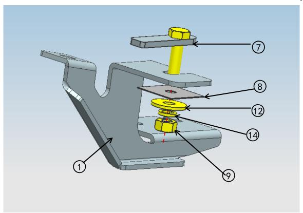
Middle Bracket (L) 3 is installed as below figure shown, Middle Bracket (R) 4 are in symmetrical installation.
