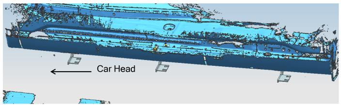
Step 3: Attach running boards on the brackets with Hex nuts M6 and Flat washers D6.
