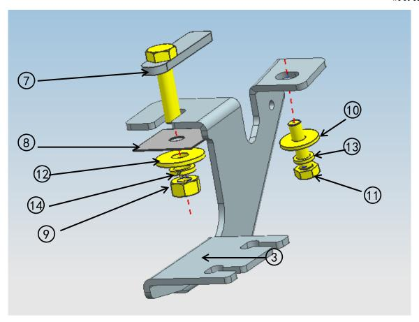
Rear Bracket (L) (5) is installed as below figure shown, Rear Bracket (R) (6) are in symmetrical installation.
