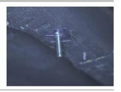
Locate and remove the hole plug in the rocker panel. Insert an M8 T-bolt plate into the opening. Slide a plastic bolt retainer over the thread of the bolt to hold the bolt in place.
