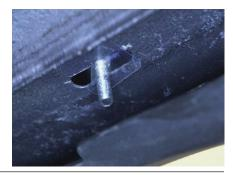
Place an L-shaped hanger bracket onto the vehicle and secure with an M8 flat washer, M8 lock washer and M8 hex nut.
