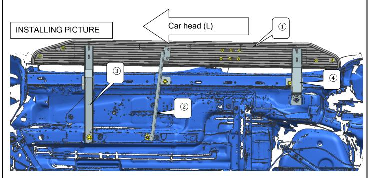
Step 1: Verify that all parts are present according to the parts list. Make a clear distinction of left and right side (driving position).
