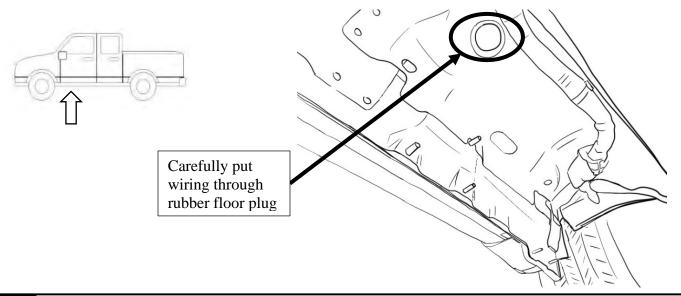
Inside the vehicle cabin, remove the driver-side front kick panel and bottom door sill plate. Peel back the carpet to access the hole where the grommet was removed. Feed the wires through.
