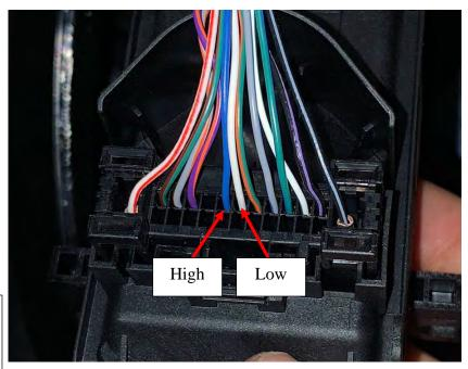
**PART B:** Confirm wires are connected in two rows (Standard OBD-II Connector). Identify the appropriate wires on back of the plug which correspond to the indicated positions on the front of the plug. Connect the Yellow (Low) and White (High) wires from the main harness (J) using the supplied wire taps (L). After successfully connecting the wires, return the module back into its place, tighten the previously removed nuts, and check that it is secure on the bracket.
