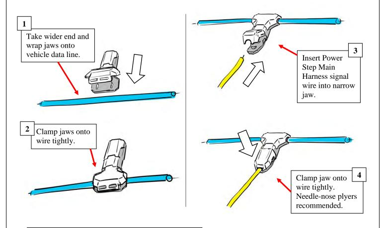
NOTE: Make sure wire is seated properly in the jaws before clamping. The wire being tapped must be centered on the "teeth" to make a proper tap.
