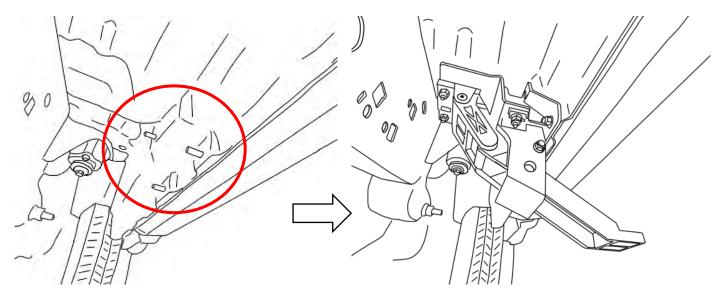
Then fasten Nylon Lock Nuts (I) and washers (H). Do not tighten all the way yet. For vehicles with e-brake cables on the Driver Side, take the rubber sleeve in the kit and slide over the brake line, near backside of the bracket assembly, to protect the line from wear. Attach sleeve to line using RTV silicone sealant.
