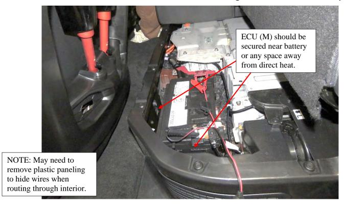
Connect the Long LED Y-harness and route the branch marked "Passenger-side" of the harness to the Passenger Side underside. **Be sure to avoid contact with any moving or hot engine components.** *It may be advisable to route along the inside of the cabin, under the carpet.* Attach and secure the main harness (J) with supplied cable ties.
