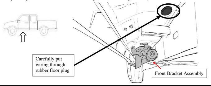
Inside the vehicle cabin, remove the bottom door sill plate and then the driver-side kick panel. Peel back the carpet to access the hole where a floor grommet can be removed. Feed the wires through.
