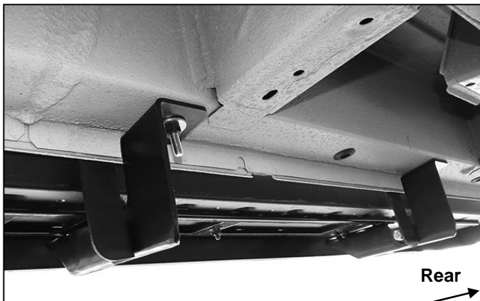
(Fig 21) Passenger side Bracket layout w-Support Brackets
