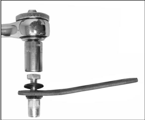
(Fig 30) Assemble Insert Tool as pictured. Turn wrench clockwise to pull/expand insert in hole
