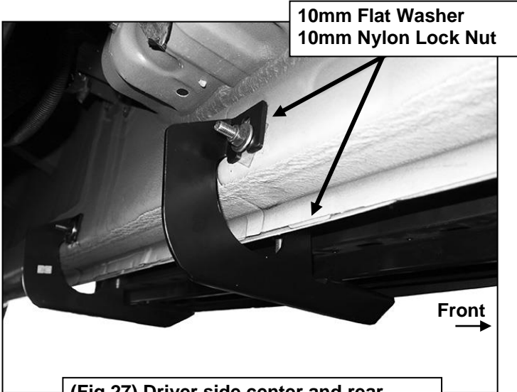
(Fig 27) Driver side center and rear Mounting Brackets completely installed
