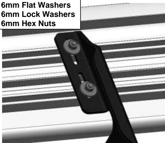
(Fig 13) Attach Running Board to Brackets
