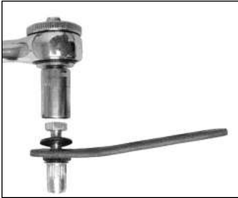
(Fig 30) Assemble Insert Tool as pictured. Turn wrench clockwise to pull/expand insert in hole
