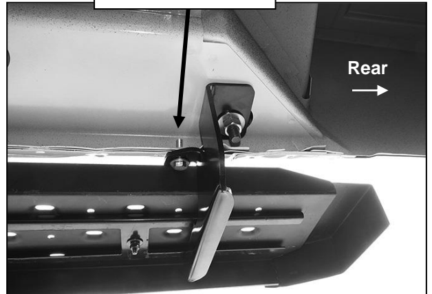
(Fig 26) Passenger/right rear Bracket installation
