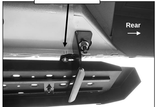
(Fig 26) Passenger/right rear Bracket installation
