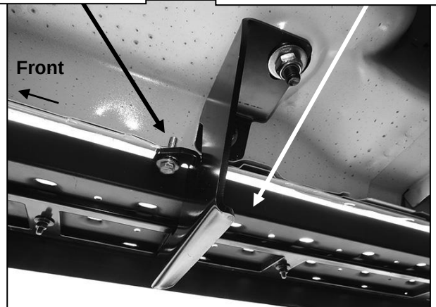
(Fig 24) Passenger/right #2 Bracket installation
