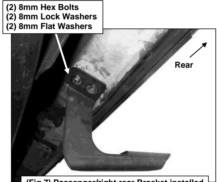
(Fig 7) Passenger/right rear Bracket installed
