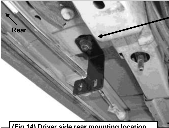
(Fig 14) Driver side rear mounting location
