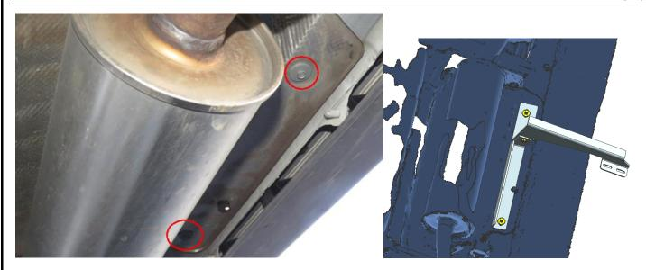
The installation of the rear bracket (L) is as follows: (see the INSTALLING PICTURE for the optional standard parts). The left and right installation methods are the same.
