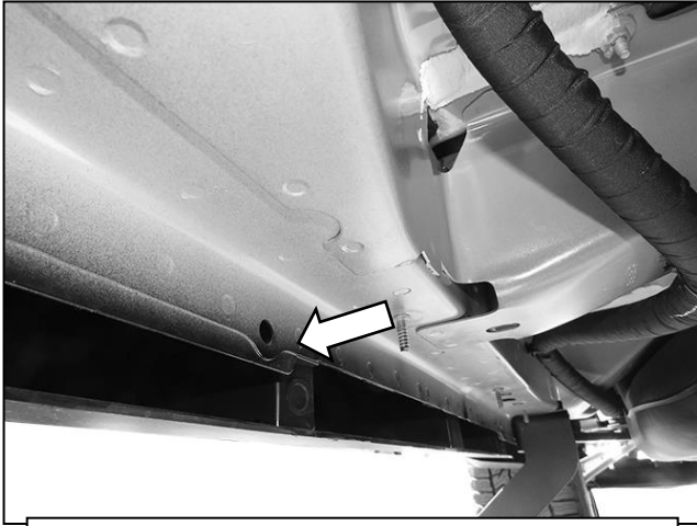
(Fig 9) Locate the Passenger/Right center mounting location. Line up the top of the Passenger/Right Center Mounting Bracket to the hole in the pinch trim. Mark the top slot for drilling. Use a 1/2" drill bit, not included
