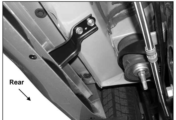
(Fig 4) Passenger side rear bracket location pictured
