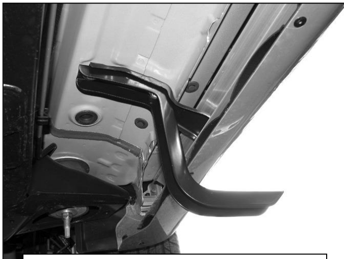
(Fig 3) Passenger side front bracket installed
