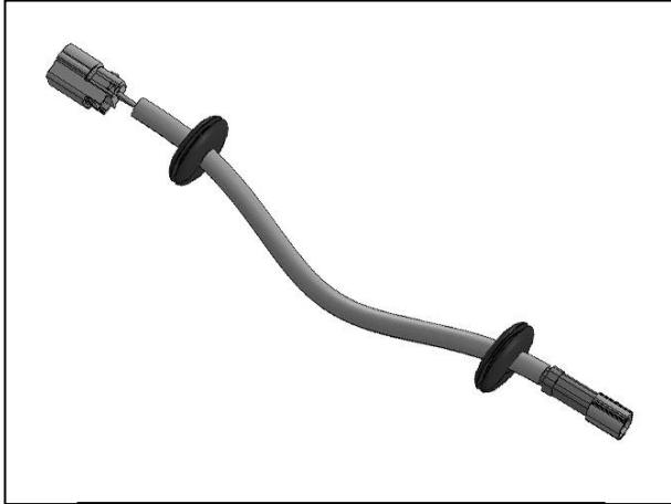
(Fig 3) Slide (2) Rubber Grommets onto Wire Harness Extension
