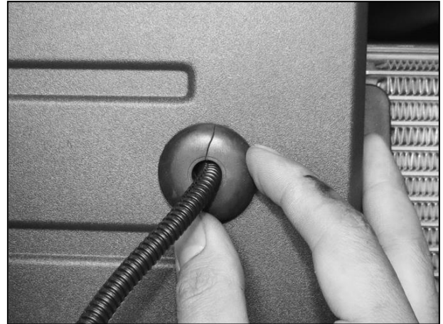
(Fig 4) Plug Harness Extension into factory harness. Push Grommet into sensor hole in bumper. Bumper pictured for example only-grommet may not fit into all bumpers
