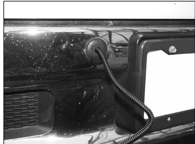
(Fig 11) Plug Harness into sensor harness
