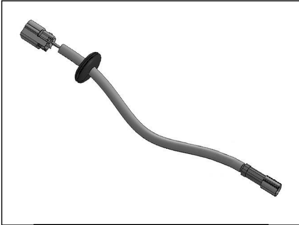
(Fig 8) Slide Rubber Grommet onto end of Wire Harness Extension
