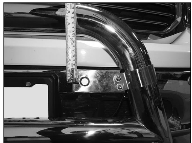
(Fig 6) 1500 models: Adjust height of Housing to approximately 4-1/4" down from bottom of top tube
