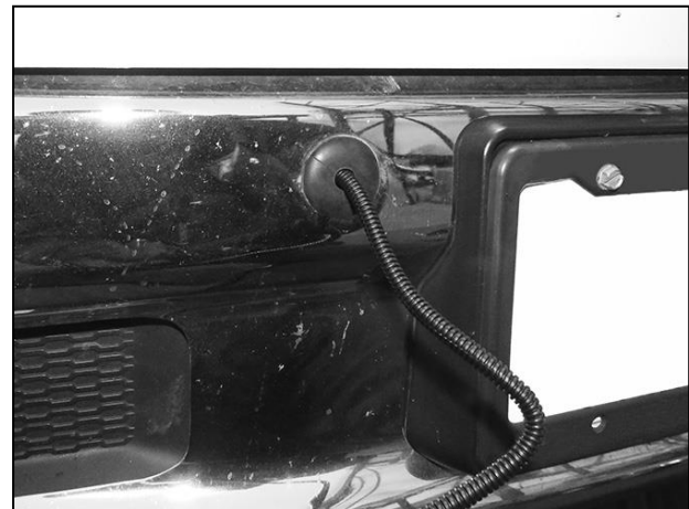
(Fig 11) Plug Harness into sensor harness
