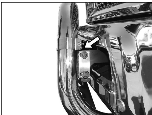
(Fig 7) 25-3500 models: Slide Housing down tube as far as possible (arrow)
