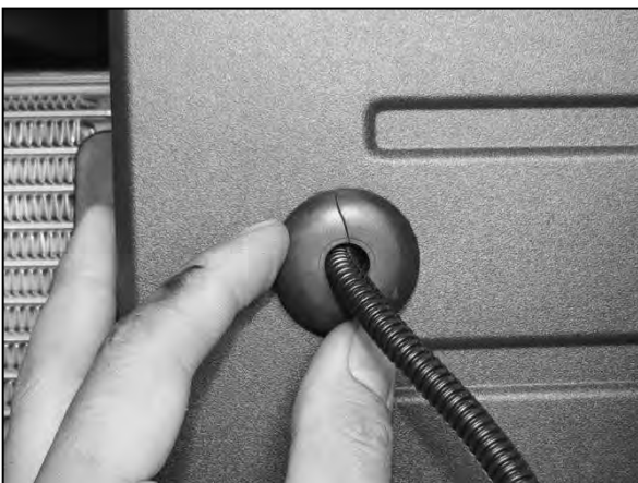
(Fig 10) Push Rubber Grommet on Harness into sensor hole (Bumper used for Example Only)
