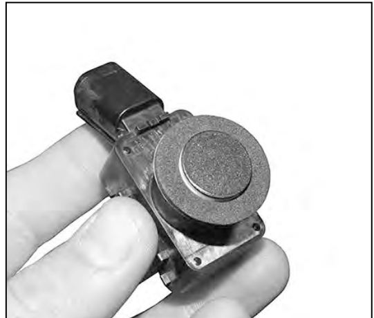
(Fig 4) Slide large Foam Seal over end of sensor
