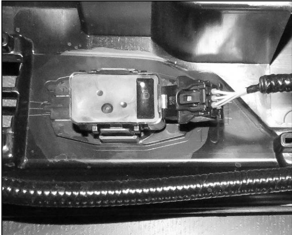
(Fig 1) Unplug and remove OE center sensors from the back of the bumper
