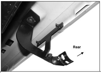
(Fig 7) Passenger/right side front Brackets installed
