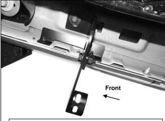
(Fig 5) Driver/left side front Brackets installed
