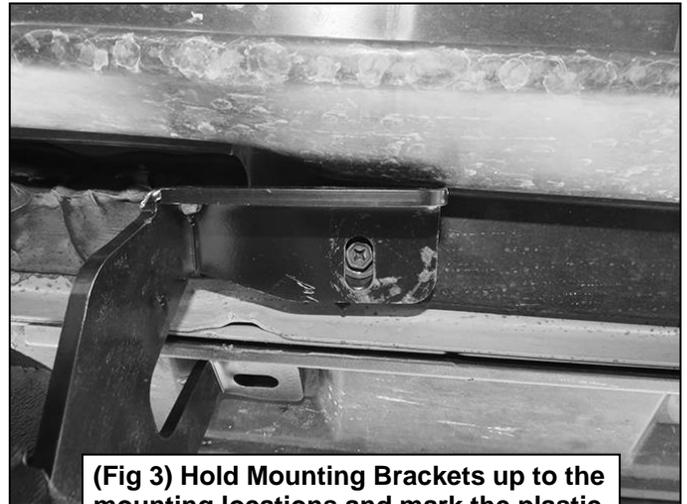
(Fig 3) Hold Mounting Brackets up to the mounting locations and mark the plastic cover (Passenger/Right Front pictured)
