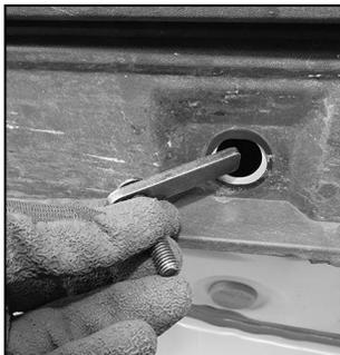
(Fig 12A) 8mm Bolt Plate
