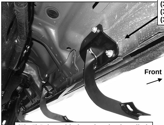
(Fig 5) Driver side front bracket installed
