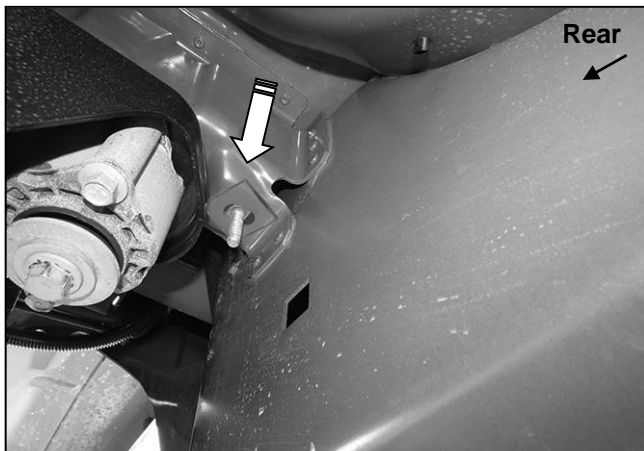
(Fig 9) Insert T-Bolt and folded Washer into oval hole. Thread second Plastic Washer onto T-Bolt
