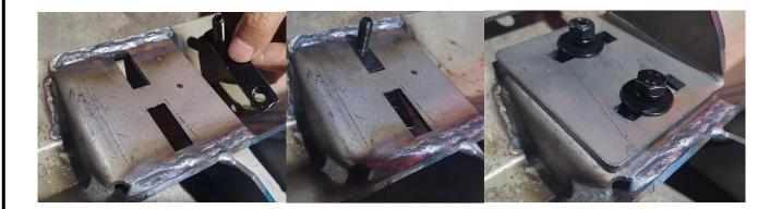
$7.\,\mathrm{Adjust}$  the front/back and up/down, then fully tighten.
