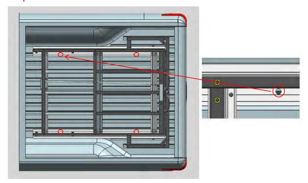
Step 8: Install the ①base of slide tray on the truck bed with hardware (19/20/21/22/23).
