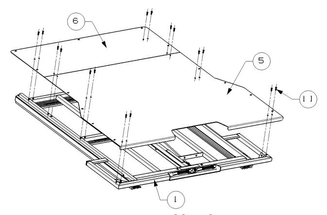
Step4: Use below hardware to install Side Plates 23 and 4 Rear Plate.
