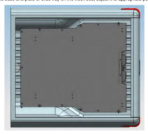
Step 6: After the position is adjusted, remove the plate of slide tray from the base in sequence as below figures shown.
