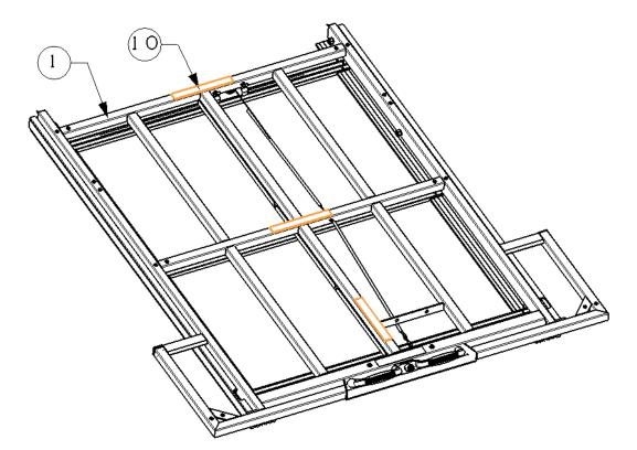
Step3: Use ①Hex Flat Head Bolts M6\_20 to install ①Base Of Slide Tray with Base Plates⑤⑥ in Page 4 of 9
