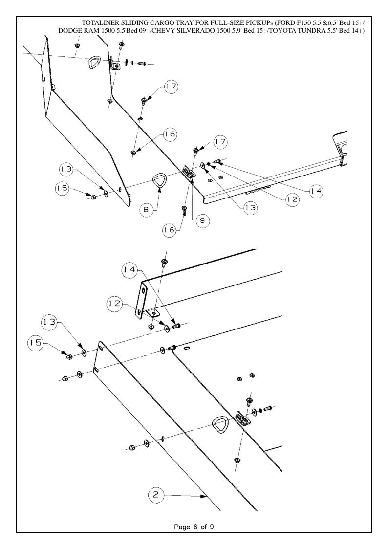
TOTALINER SLIDING CARGO TRAY FOR FULL-SIZE PICKUPs (FORD F150 5.5'&6.5' Bed 15+/DODGE RAM 1500 5.5'Bed 09+/CHEVY SILVERADO 1500 5.9' Bed 15+/TOYOTA TUNDRA 5.5' Bed 14+) Step5: Put the base and plate of slide tray on the truck bed, adjust it to appropriate position.
