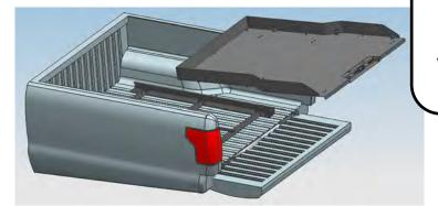
Press and hold the button, and pull the plate out, you can remove whole plate when it is near the end of the base.
