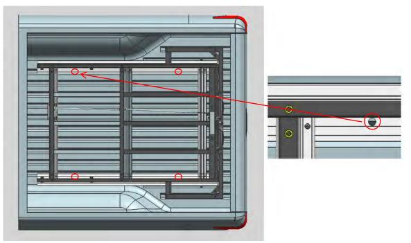
Step 4: Install the base of slide tray (1) on the truck bed with hardwares (2)(3)(4)(5)(6)
