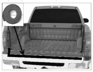
② Another seal put on the clamp to avoid any scratches happen while touching the car body.
