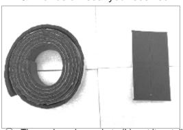
① The seal on above photo (L), put it on tailgate door. (As the photo shows below)
