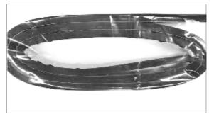
Put on this seal on bulkhead if it is not flat, to make the bulkhead can full contact with the tonneau cover.
