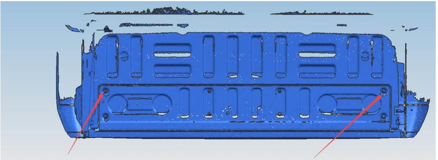
Step 2: Put the seat mat on tailgate and adjust the seat mat in appropriate location, install it with factory bolt and lock tighten.
