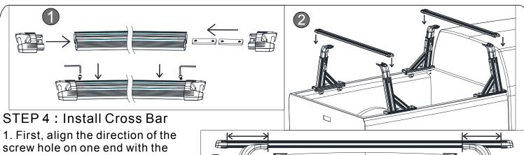
1. First, align the direction of the screw hole on one end with the graduated surface. Install to the slot corresponding to the cross bar and insert to the bottom. At the other end, install two M8 cross bar screw square gaskets into the slot marked with a scale on one side. Then install the cap into the cross bar slot. The installation method is the same as the other side. Finally, install M6 screws and fasten them with the corresponding M6 wrench.
