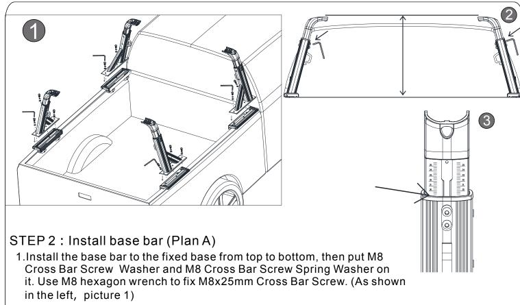
2. The base bar can be adjusted according to different vehicle types. Loosen the screws on both sides of the base bar with M10 hexagon head wrench, then adjust according to the required height. There is a scale mark on each base bar. Adjust each base bar to the same scale and tighten with a wrench. (As shown in the right, picture 2, 3)
