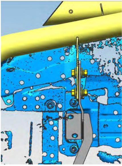
Step 3: Install the bar body on the bracket and adjust the mounting position of the bracket according to the position of the bar body
