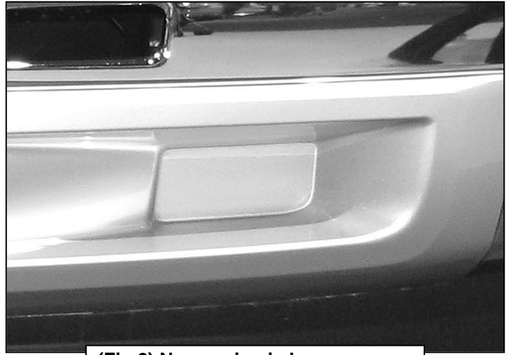
(Fig 2) No opening in bumper cover
