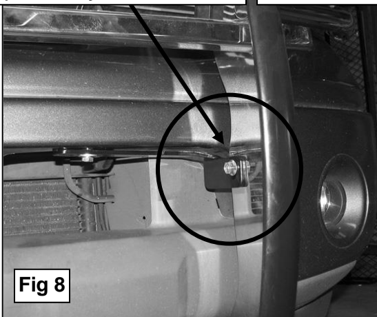
05-08 driver side Top Bracket installation pictured
