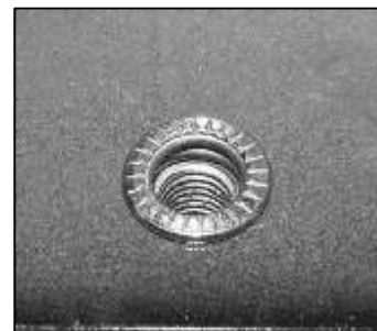
(Fig 6) Example of fully installed 6mm Insert.
