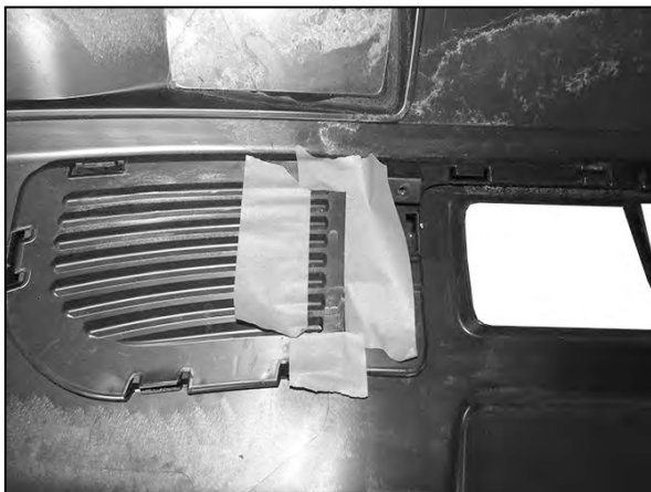
(Fig 19) From behind the bumper mark the indicated area with tape. Use a hacksaw or sharp knife to make small cuts to clear Brackets
