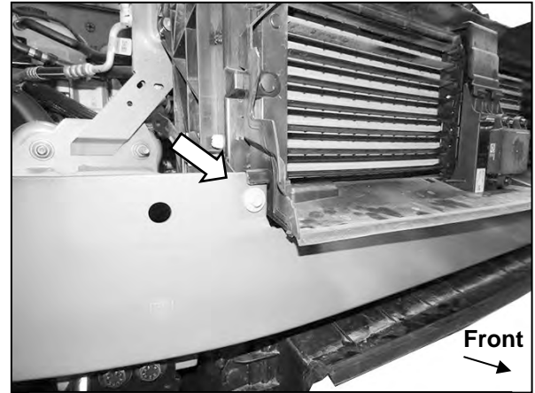
(Fig 18) Remove the bolt in the upper crossbar (passenger/right side pictured)
