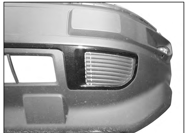
(Fig 20) Marked area pictured for example only. Use a hacksaw or sharp knife to make small cuts to clear Brackets.
