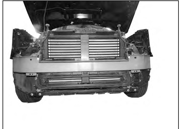
(Fig 10) Carefully remove the bumper cover assembly and place it on a clean, soft surface
