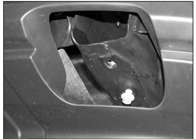
(Fig 2) Tow hook model pictured with factory nut plate in frame channel
