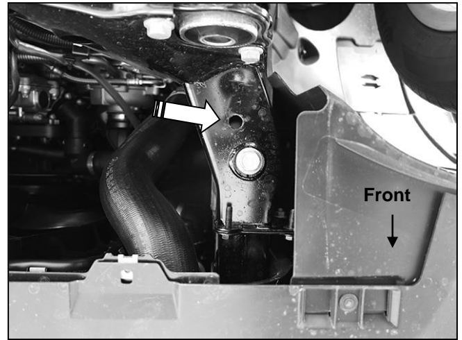
(Fig 2) Locate round hole in bottom of frame (arrow). Insert 8mm Bolt Plate into factory hole in frame rail.
