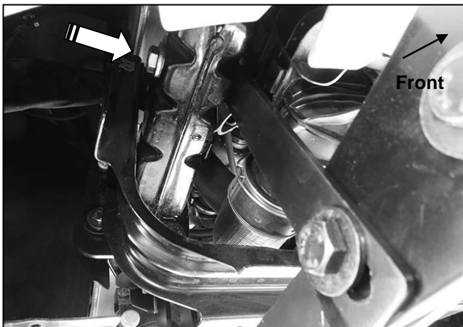
(Fig 8) Passenger/right Support Strap attached to bumper bracket (arrow-pictured from below)
