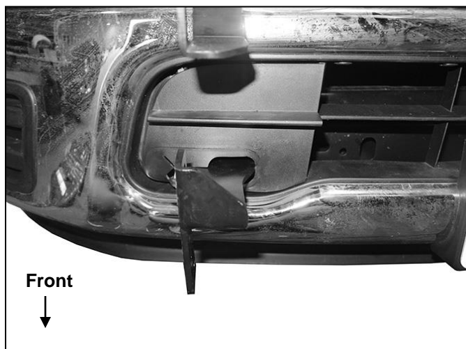
(Fig 3) Slide Passenger/right side Bracket through opening in cover for tow hook
