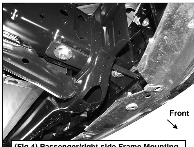
(Fig 4) Passenger/right side Frame Mounting Bracket installed (pictured from below)
