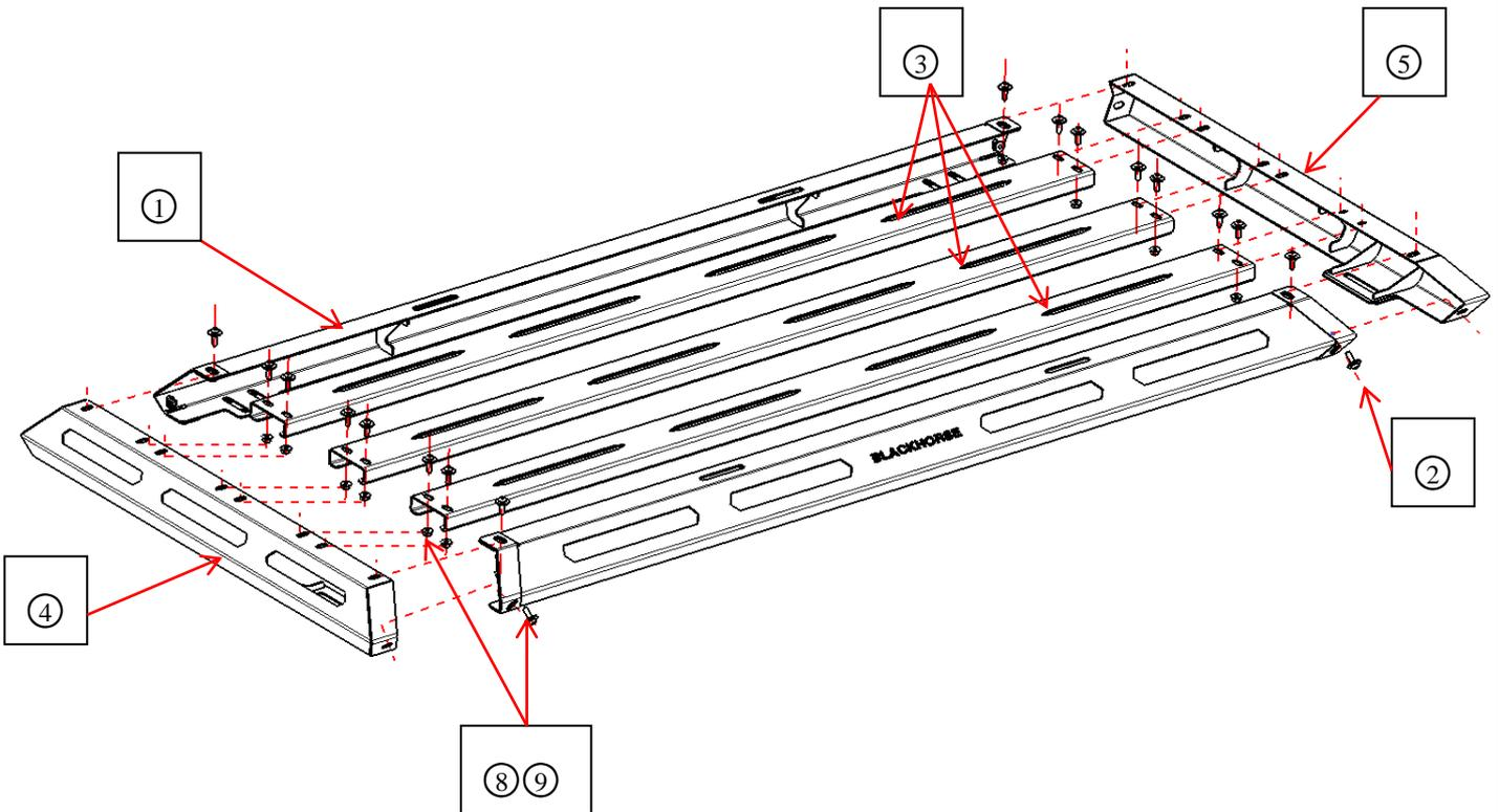
**Step2:** Connect the roof basket with ARMOUR II roll bar with ⑥connecting bracket, then Lock all the standard
