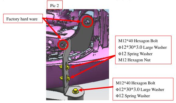
Step 4: Check if all hard ware are installed and then fasten all to complete the installation.
