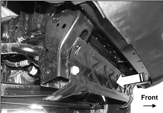
(Fig 1) Remove splash guard and bracket (arrow)
