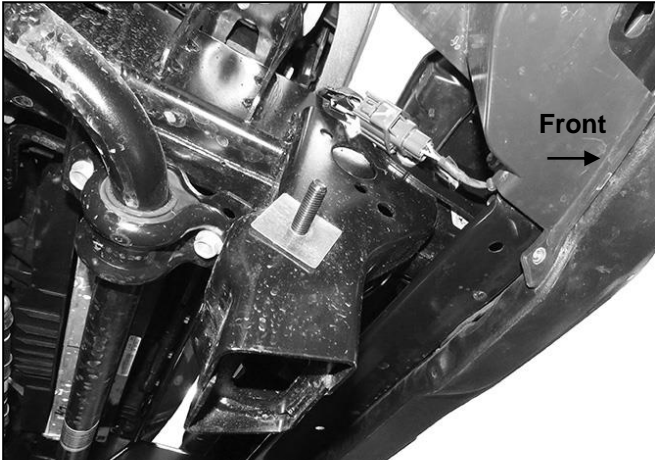
(Fig 3) Use Retainer to hold 10mm Bolt/Nut Plate
